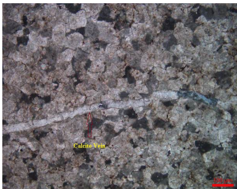
Pmg – 3: Photomicrograph showing calcite vein intrusion within dolostone as seen under crossed nicols. Specimen No.: MK-PET-04 Magnification: 100X
