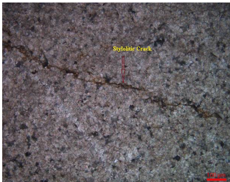
Pmg – 1: Photomicrograph showing ferruginous filling along stylolitic cracks in dolomite as seen under crossed nicols.
