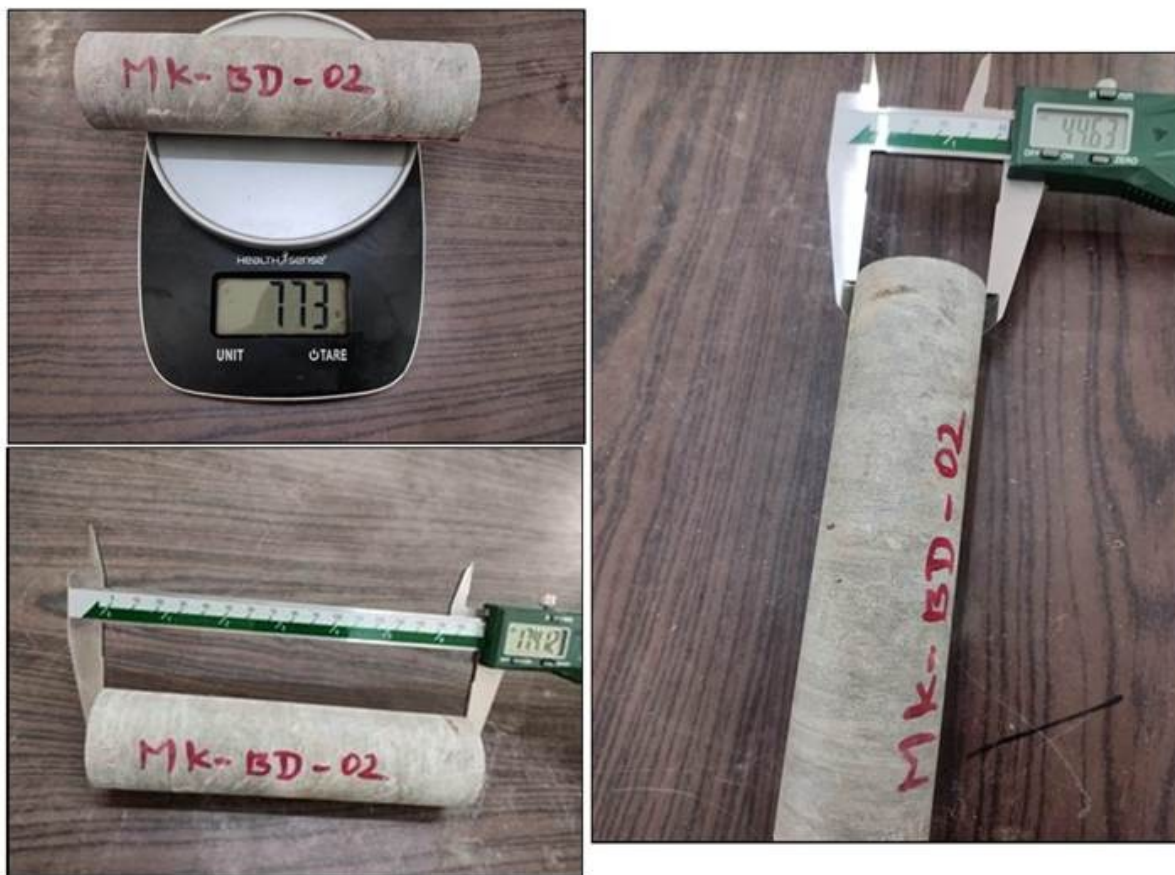
Figure 9: Photographs showing procedure of determination of length, diameter and weight of sample number MK-BD-02 for bulk density calculation
