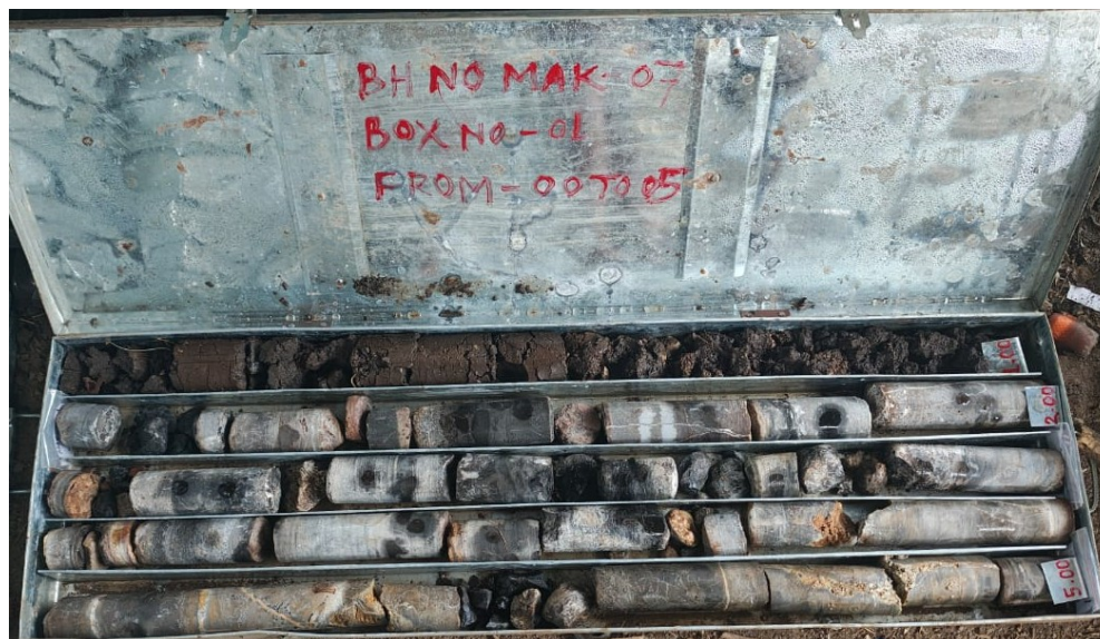
Figure 1: Photograph showing cores of limestone zone from 1m to 5m in MAK-07
